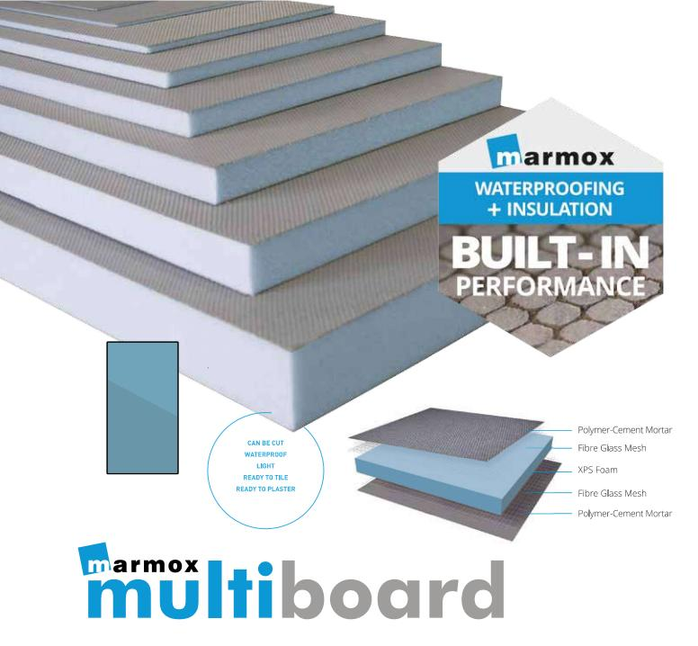
Marmox Multiboard is a lightweight, high-performance tile backer board, used for waterproofing, dry-lining and thermal insulation, offering the best long-term adhesion in its class. Marmox Multiboard consists of a core of extruded polystyrene bonded between layers of fibreglass reinforced polymer concrete.
